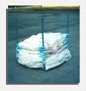
Place loops over two poles and lay the bag flat on the pallet. Place the lift loops of the next bag over the opposite two poles. Alternate sides with each bag. Stack bags to the top of the rack, minimum of 50 bags.
