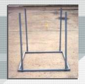
Place pallet in rack, up to a 42" x 48" pallet. Place cover bag on pallet and lay flat. Make sure the edges of the bag are accessible.
