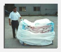
Compress the bags using a forklift, then remove the poles. Pull the cover bag up around the bags and tape it closed. Strap the bags to the pallet using three straps.
